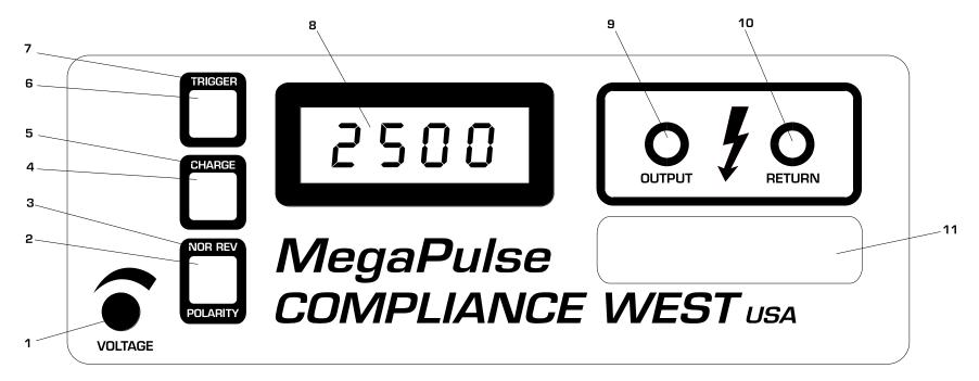
Figure 2. Controls, Indicators, Connectors – MegaPulse series Front Panel
