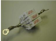
12. Connect the measuring instrument across the current shunt, keeping in mind that the Return lead is referenced to ground.
