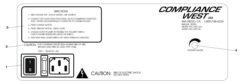
Figure 3. Controls, Indicators, Connectors – MegaPulse series Rear Panel
